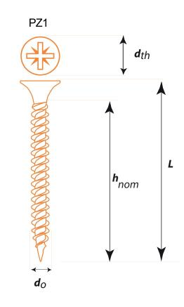
The FFX Hitech Double CSK Head Multi-Purpose Screw. Hitech case hardened Multi-Purpose screws, with a double countersunk pozi recess head, for improved head shear resistance. Sharp 28° point enables easy penetration into all recommended substrates
